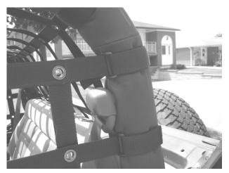
The four straps at the top of each side will connect to the top piece after you have installed the overhead piece.
