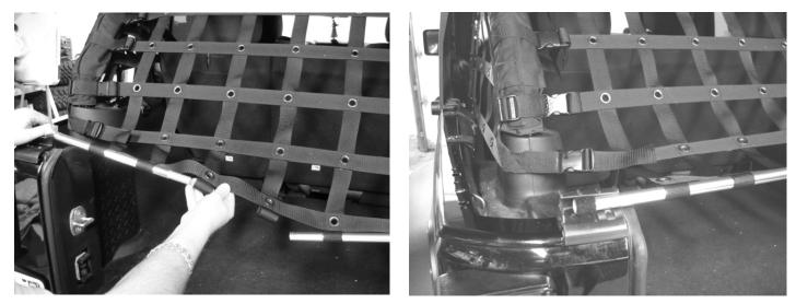
The strap at the very top of the rear piece wraps around the top of the vertical roll bar comes toward the outside wraps back around and connects into the ladderloc clip. See photo
