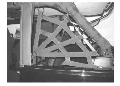
Any excess straps that hang out can be tucked in under itself. Adjust and tighten straps as needed to even out the net so it is positioned properly. Your net comes with a 3 year warranty against manufacturing defects. Cuts, abrasions, sun faded items are not covered under the warranty.
