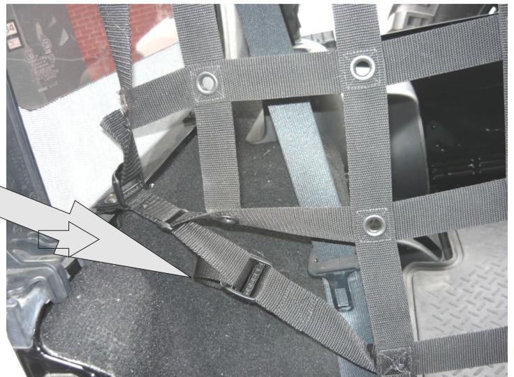
Wrap the strap at the top around the side roll bar and connect it to the ladderloc on the adjacent strap. The last step is now to connect the bottom of this strap to the ladderloc that you attached to the truck in the last step
