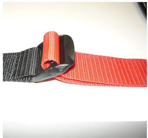
Next attach the ladderloc and loop with the grommet strap to the hardtop bolt. The ladderloc is on top and the loop hangs below. We have provided a longer bolt if the existing hard top bolt is to short. We have also provided a nut and washer for none hard top owners.
