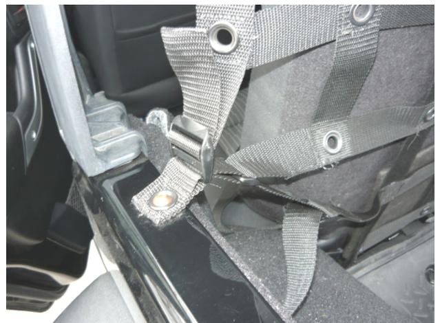
Attach the horizontal strap through the loop and connect to the ladderloc on the strap below it as shown.
