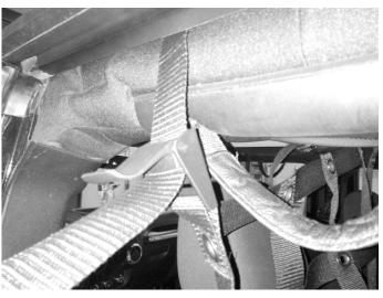
The long straps at the bottom pull down and wrap underneath the front seat seat brackets as shown. The JK and JKU have different style seat brackets. As seen in the two photos. The straps come back up and connect into the lower Cam buckle.
