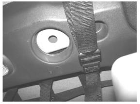
The two straps that run out horizontilly at the top go over top the roll bar and come out around the side. These connect into the cam buckles on the net. (see Photo). Tighten up both sides and postion the net so everything is centered and hanging evenly.
