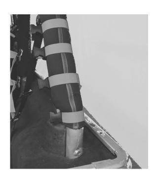
The next step is to install the male side of the side release buckle on the rear net section as shown. 4 on each side. Snap these buckles into the female side you just installed on the roll bars as shown below. Tighten the straps evenly along each side until you get a uniform look.
