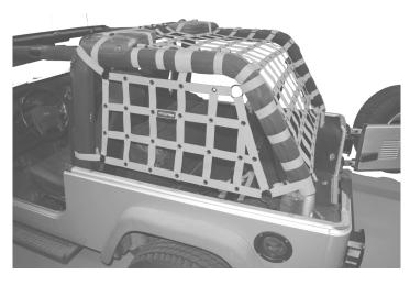
There is one last strap on the side at the top that wraps around the roll bar. Repeat this procedure for the other side.
