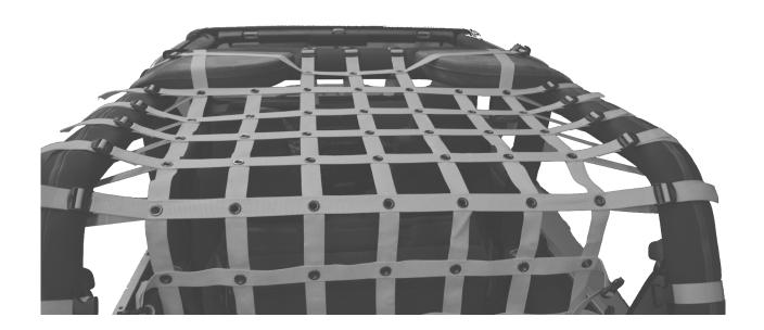
Start with either side next. There is a left and right side net. The dirtydog logo faces outward. There are 4 rings on each side. You will use the 4-29 inch straps to tie this piece onto the roll bars as shown in the photos below. At the bottom of each side there are 2 J hooks that clip to the underside of the tub.
