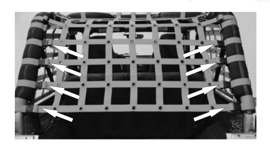
Install the rest of the straps around the roll bar as shown in the picture below
