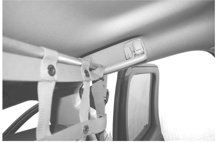
Step 4: Connect top strap around roof top grab handles and feed into ladderloc. be sure to run the webbing through the top loop on the net first.
