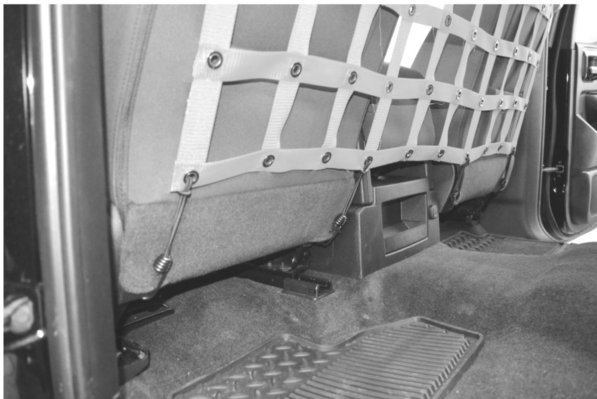
Step 6: Attach the side straps to the grab handles at the doors as shown. Tighten equally on both side. Your pet divider is now installed.
