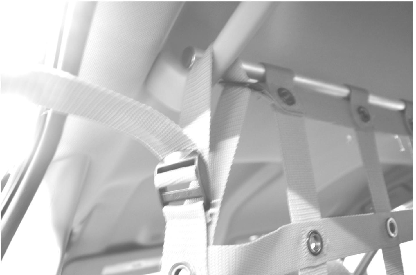
Step 5 Attach the bottom shock cords to the under side of the seats as shown.
