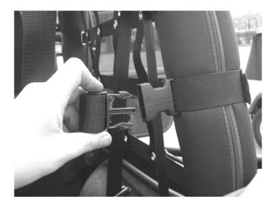
The last strap at the very top wraps around the roll bar and comes out the side to attach to the buckle off the side
