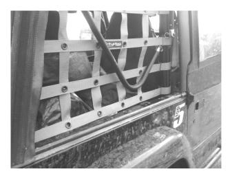
Rear section installation. Start at the back with the rear buckles. Attach all ten. Tighten and adjust as necessary. Finish by installing the balance of the straps along the top. There are 3 more straps at the top that install on the roll bar
